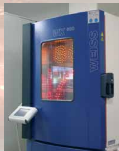
In-house climate testing of the boards
